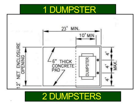
b. Double (two 3, 4, 6, or 8-yard) dumpster enclosure shall be no less than 10 feet deep x 24 feet wide. The minimum width of the gate or doors shall be no less than the enclosure opening, and they shall open 180°.
